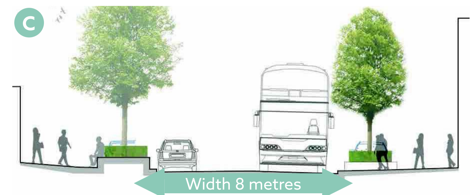
Typical proposed carriageway width. Two cars and a bus could still pass with ease.
